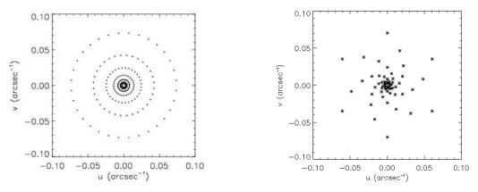
Figure 1. Sampling of the spatial frequency plane. Left: RHESSI. Right: STIX
